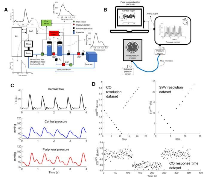
**Figure 1.** (A) Schematic diagram of the mock circulatory loop (MCL). (B) Schematic diagram of the setup for evaluating a bench pulse contour CO monitoring system. (C) Example flow and corresponding pressure waveforms produced by the MCL. (D) Normovolemic datasets for quantifying three dynamic attributes of pulse contour CO monitoring systems.
