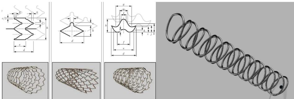
Figure 1: Mesh geometry variations of intricate patterns (left) and simple loop coil (right)
